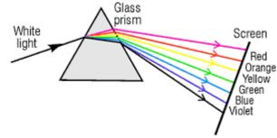
Fig. : A glass prism splits the white light into seven colors.
